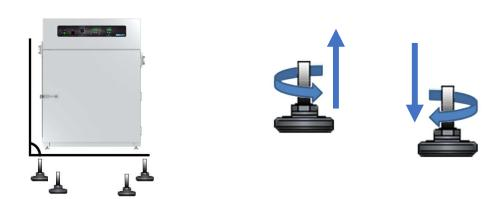
**Note:** To prevent damage when moving the unit, turn all four leveling feet so that the leg of each foot sits inside the unit.
