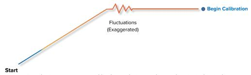
Required temperature stabilization period operating undisturbed with the incubator doors closed.
