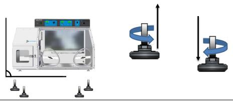
**Note:** To prevent damage when moving the unit, turn all 4 leveling feet so that the leg of each foot sits inside the unit.
