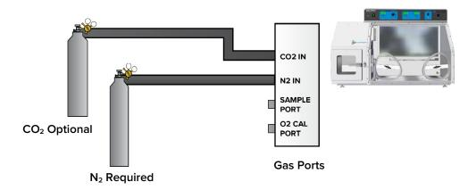
Match the correct gas regulator type to the correct gas type. A  $CO_2$  regulator should always be used for  $CO_2$  supplies, etc.
