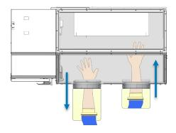
Placing only one arm all the way in the chamber reduces the volume of displaced atmosphere.
