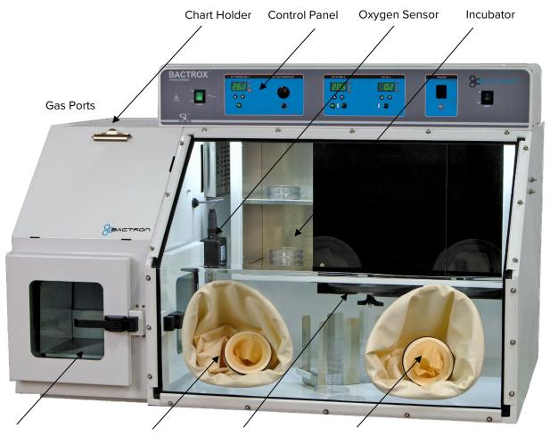
Pass Box Arm Port with Sleeve Arm Port Door Storage Arm Port with Sleeve
