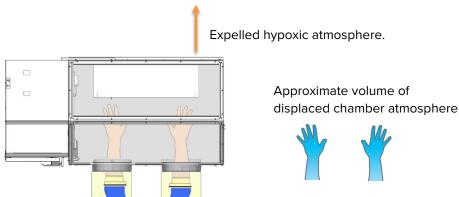
Use the following techniques to reduce displacement and gas usage while working in the chamber.
