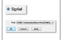
6. Connection: If using Tera Term, the emulator should start logging data from the BACTROX-2 once every minute if the correct com port was chosen. If the emulator is not logging the data, perform the following steps.
