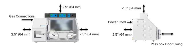
2.5 inches (64 mm) minimum clearances are required for unobstructed airflow and cooling.
