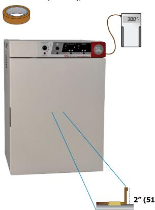
**CO<sub>2</sub> Calibration**: A CO<sub>2</sub> calibration may be performed during the temperature calibration so long as the chamber door and access port remain closed and sealed.
