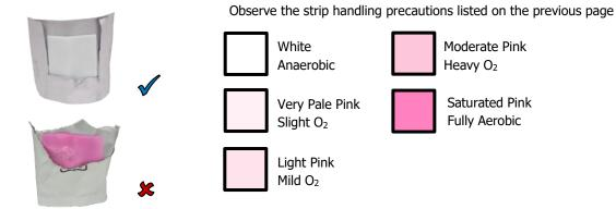
4. If the strip remains white, the chamber is anaerobic. Exit the chamber using the steps in the Exit the Chamber procedure on page 55. **The verification procedure is complete**.
