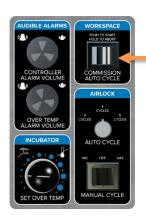
Briefly, press the Commissioning Cycle button on the side shadowbox control panel.
