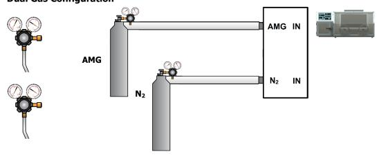
Do not start a flow of gas to the BACTRON at this time for either configuration.
