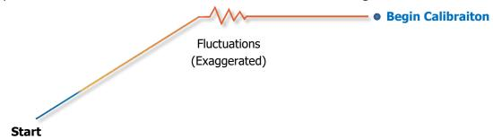
Required temperature stabalization period operating undisturbed with the incubator doors closed.
