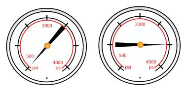
The supply gauge (right) will jump from zero ( 0 ) to showing the current gas supply pressure level.
