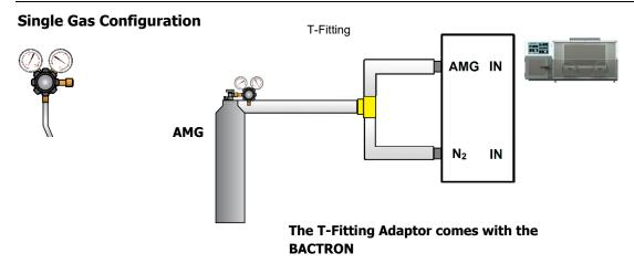
Failure to connect the T-fitting to **both** the AMG and Nitrogen In ports will interfere with the airlock auto cycle. The Nitrogen in port must always be connected to either the AMG or an  $N_2$  supply.
