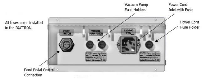
**Figure 3: Power Supply Panel**All Units (Located on back, behind the airlock)
