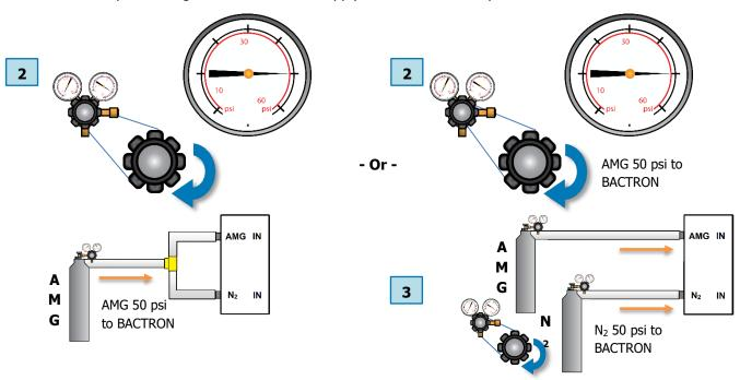
3. **Optional:** Open the Nitrogen regulator valve to supply an N<sub>2</sub> flow of 50 psi to the BACTRON N<sub>2</sub> port.
