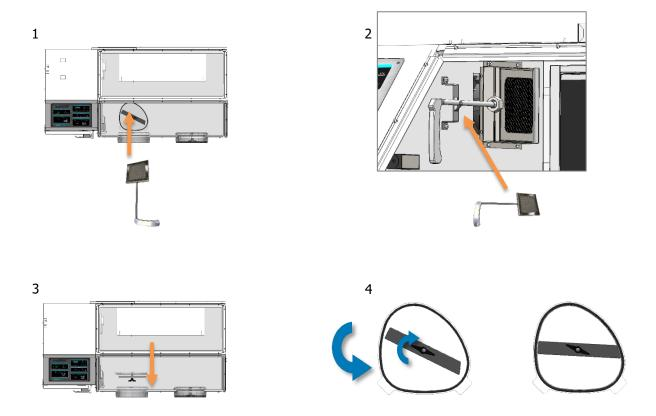
See page 29 for instructions on **properly closing and latching the arm port door**. Whenever the chamber is anaerobic, scrubbers should be introduced and removed through the airlock.
