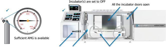
Both airlock doors are closed and latched Manometer is filled Arm port doors are closed and latched
