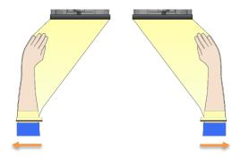
This position prevents the collapsing sleeves from pulling your hands into the arm port doors during the vacuum down cycle phases. It also keeps the sleeve material tight, helping to obtain a complete evacuation of the sleeves.
